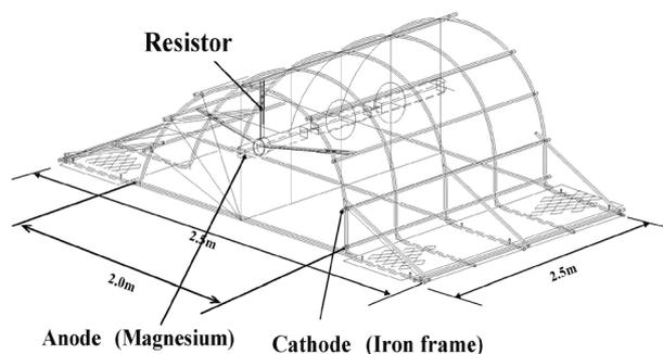
**Fig. 3** Framework of the cage structure for the undersea experiment
