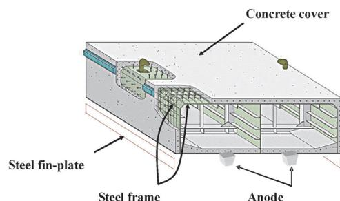
Fig. 1 Photograph and schematic representation of the hybrid-type pontoon installed at Taketomi-higashi Port
