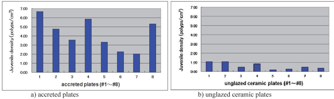
**Fig. 5** Number of coral polyps on the surface of settling plates under different current densities a): for accreted plates; b): for unglazed ceramic plates: plates #1 & #2, null current; #3 & #4, 10 mA/m<sup>2</sup>; #5 & #6, 50 mA/m<sup>2</sup>; and #7 & #8, 100 mA/m<sup>2</sup>
