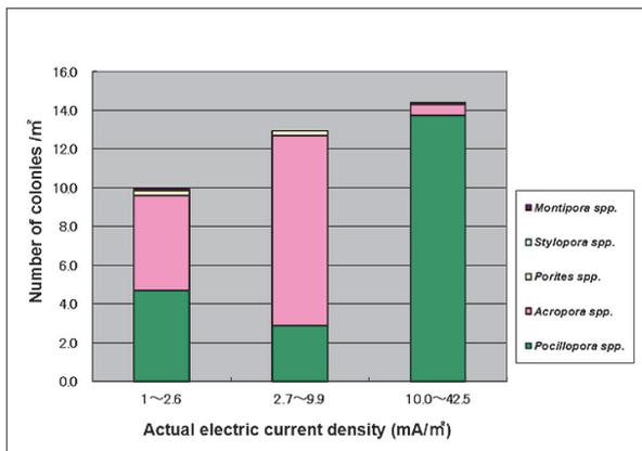
**Fig. 2** Electric current density and number of coral colonies on the pontoon surface
